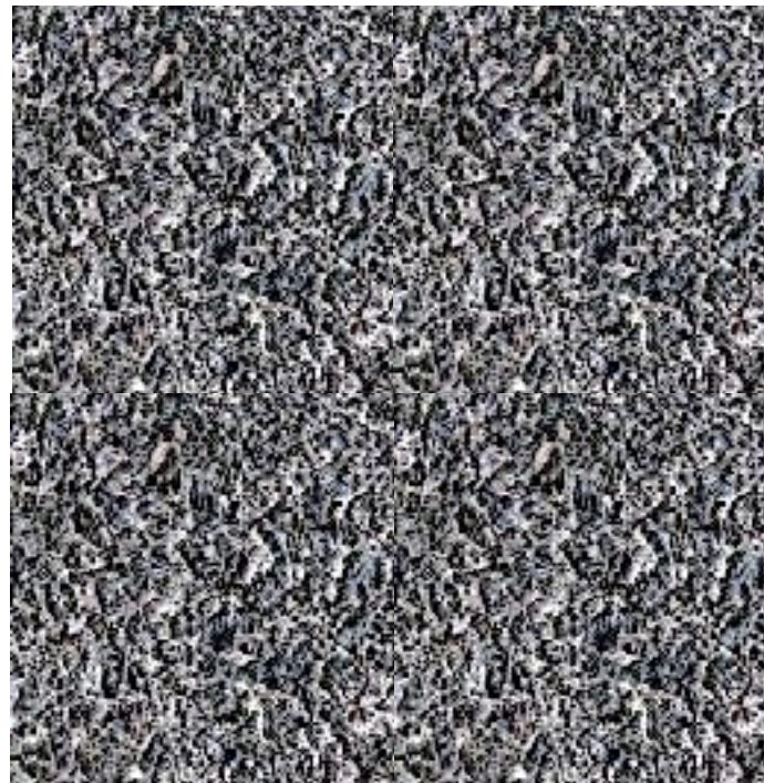
exposed surface (the cement glue is washed off)
